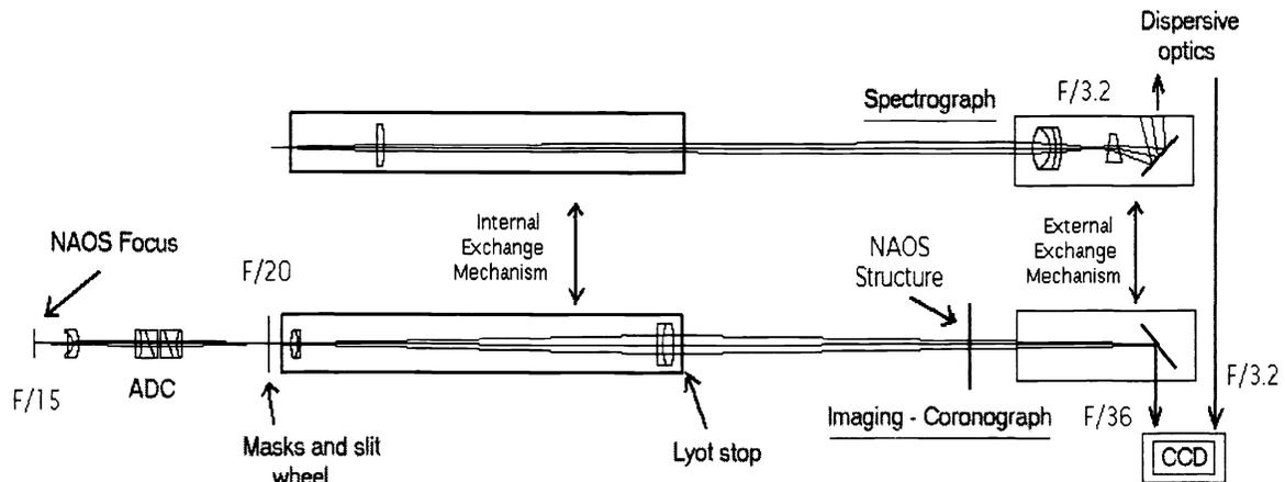
**Figure 2.** The relay system from the AO focus to either the AVES spectrograph or the imager/coronagraph.
