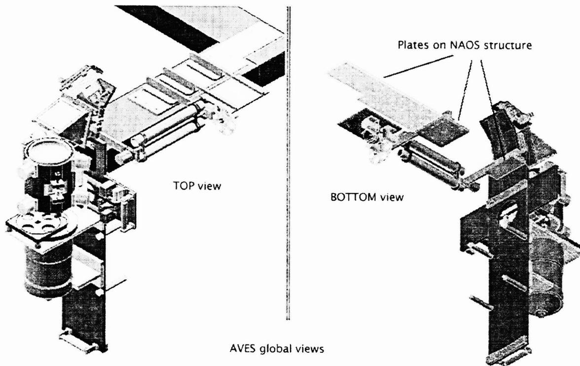
Figure 3. The mechanical structure of the AVES-IMCO instrument
